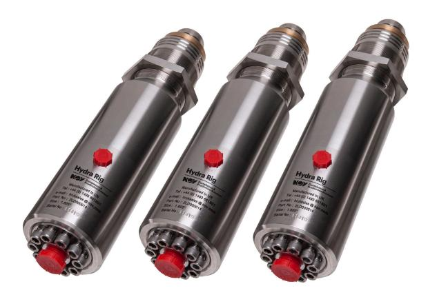
Our cryogenic cold ends are designed to complement our NP-200 power end but are compatible with most other manufacturers' power ends using a 1.38-in. stroke. These are available in a range of sizes from  $1\frac{1}{4}$  to 2 in. and working pressures up to 15,000 psi.
