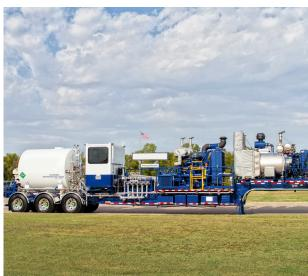
Our direct-fired trailer-mounted nitrogen pumping units provide a platform for super high-rate flows, and its high-volume capabilities allow for reduced equipment requirements on large volume jobs.
