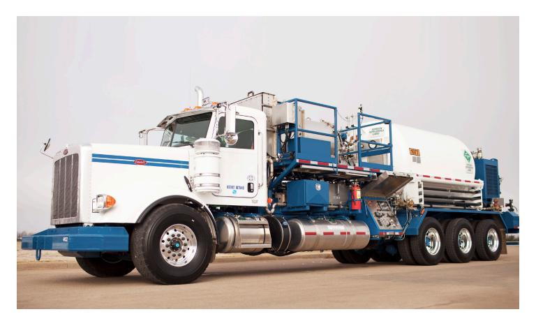
Designed with a condensed footprint for hard-to-access locations, our direct-fired chassis-mounted nitrogen units are ideal for fracturing applications or any situation where a high flow rate is required. They come standard with a main engine, transmission, reduction/drop box, triplex nitrogen pump, nitrogen boost pump, direct-fired vaporizer, hydraulics, liquid nitrogen storage tank, and necessary piping and controls. These models can be built on any major brand of truck chassis.
