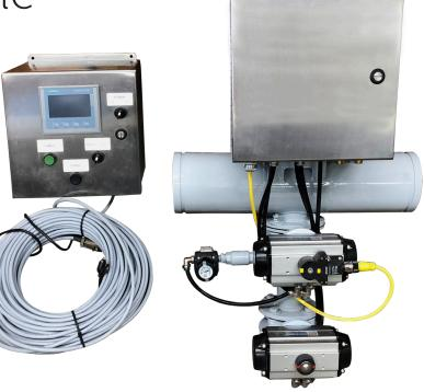
The Wilco™ automatic sample catcher system is designed for easily removing a representative sample of dry material as it passes through pneumatic process piping. Our system consists of the sample catcher mounted to the piping and a controller that can be remotely mounted, such as in a control room. The easy-to-use electronic controller allows the operator to take a single sample or start and stop the sampler with preset timing modes for small, medium, and large blends.
