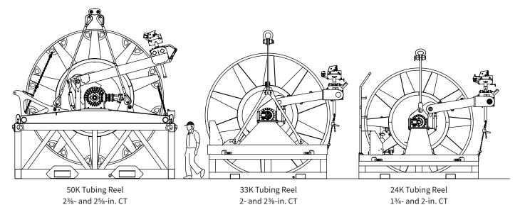
Our tubing reel product line consists of reels sized to meet different applications, tubing sizes, and capacities. The 50K is currently the largest, suited for long strings, large units, and milling. The 33K and 24K are sized for medium and small strings where transportation limits are more restrictive. Contact your NOV sales representative to determine the right reel for your operation's needs.
