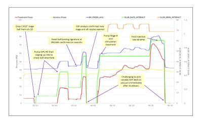
Ball displacement, sleeve opening, and acid stimulation plot
