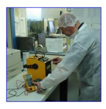
Procon Engineers are trained to maintain and calibrate temperature controls, and we carry a wide range of test equipment including hot baths, TP100, mV & mA simulators. Our scope includes equipment such as:
