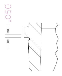
Figure 20 MACHINING OF VALVE SHOULDER
